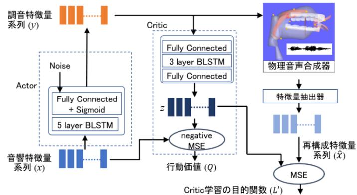
図 2 Hybrid Auto-encoder based Physical Speech Synthesis system.
