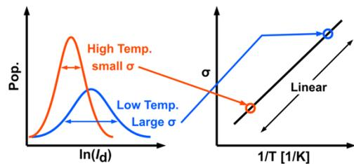
$$\sigma(\ln(I_d)) \approx \sigma \left( \frac{V_{th}}{n} \right) \frac{q}{kT} \propto \frac{1}{T}$$
